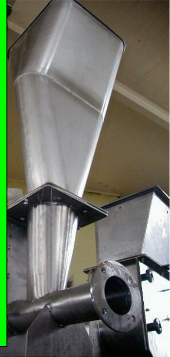
Even better results can be achieved if the end walls actually diverge whilst the sidewalls converge steeply. This technique relaxes the confining stress in one plane – coined “**Sigma2 Relief**” by **Ajax Equipment** – and it facilitates an even narrower slot outlet. **AJAX** supplements this method with screw feeders that offer fully progressive extraction along the length and width of the slot.
